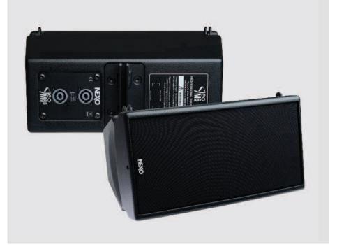
The GEO M6B is a low and mid-frequency partner module to the GEO M620, for applications which demand more powerful reinforcement, such as live music. With one 6.5"  $8\Omega$  long-excursion driver, the M6B weighs just 7.6kgs and shares the same physical footprint as the M620 allowing the cabinets to be arrayed together in the same column. Featuring a flare-shaped port tube to increase low frequency efficiency and linearity at high power, the M6B offers a usable range @-6dB of 70Hz-1kHz.
